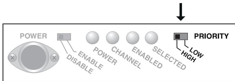
This switch allows you to set the priority of the Barr CHANNEL device to HIGH or LOW.
