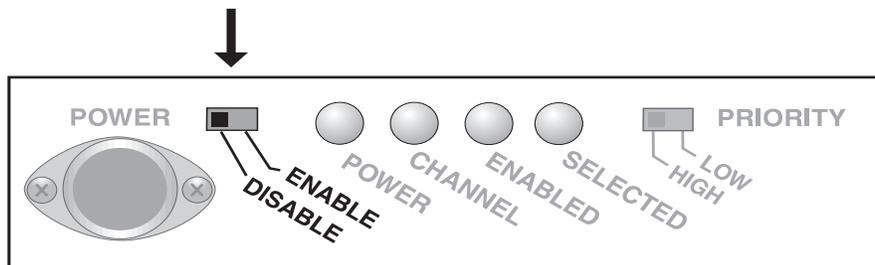
Use the switch to connect the computer to or disconnect the computer from the channel.
