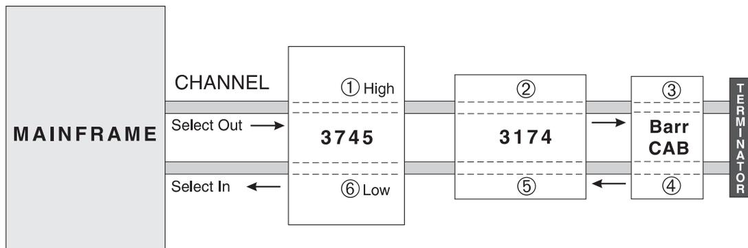
The mainframe raises Select Out when a channel device signals that it wants to begin communications. The mainframe signal passes from channel device to channel device along the Select Out line and then returns from channel device to channel device along the Select In line. A channel device that is ready to begin communication with the mainframe will not pass the Select signal to the next channel device until it has completed communication with the mainframe.
