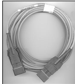
7-meter (23-foot) fiber-optic cable for connecting the adapter to the CHANNEL-IN (ES) device
