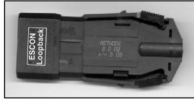
Loopback plug for testing the cable and adapter
