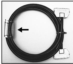
The adapter test plug comes strapped to the cable connecting the CHANNEL adapter and CAB.
