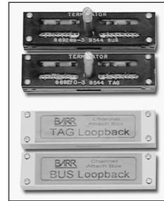
The Diagnostic Tools Bag contains the CAB terminator plugs, loopback test plugs, and instructions for installing the plugs on the CAB.
