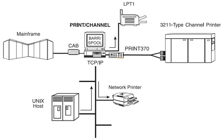
**Figure 1-2.** PRINT/CHANNEL with BARR/SPOOL, PRINT370, and TCP/IP.
