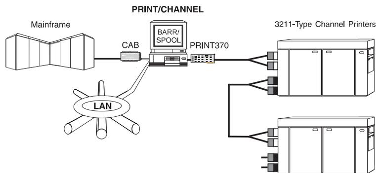
**Figure 1-1.** PRINT/CHANNEL with BARR/SPOOL and PRINT370 allows you to share mainframe printers with the network.
