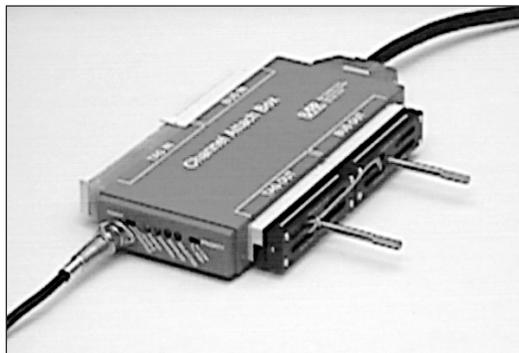
CAB with terminator and loopback test plugs installed.
